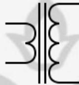
Gambar 2.39 Simbol transformator step-up
