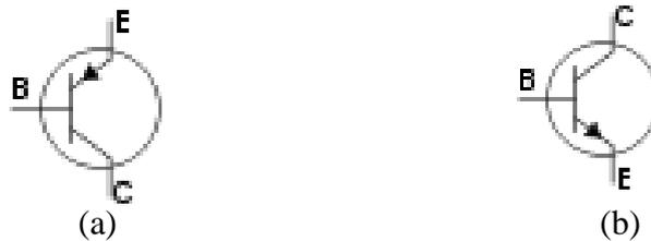
Gambar 2.38 (a) transistor PNP (b) transistor NPN
