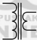
Gambar 2.40 Simbol transformator step-down
