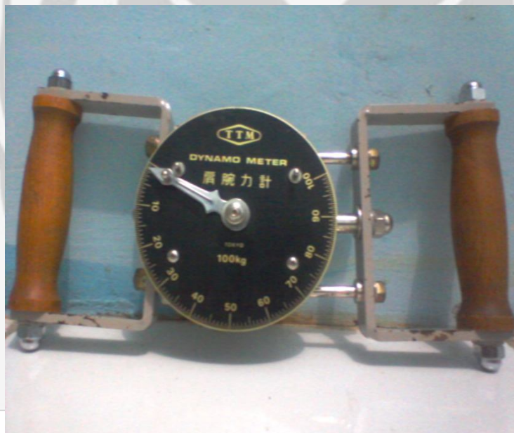
Gambar 8 : push and pull dynamometer
