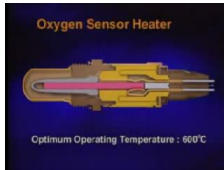
Gambar 5. Temperatur optimal O_2 sensor
