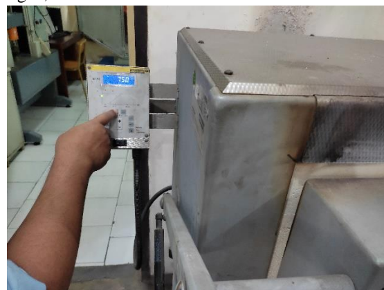
Gambar 4. Pengaturan temperature furnace
