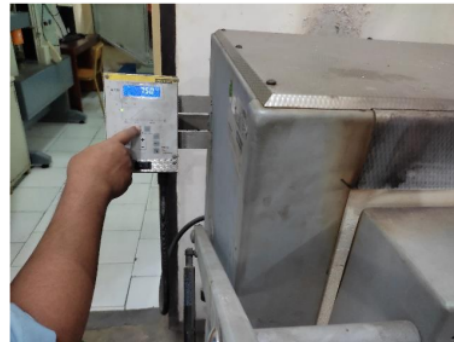
Gambar 2. Pengaturan temperature furnace
