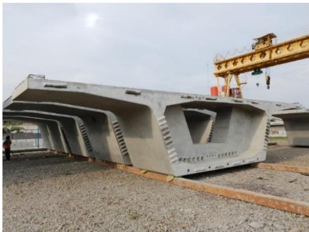
Gambar 2.4 Gelagar kotak (*Box girder*) (PT Jaya Beton Indonesia, 2016).
