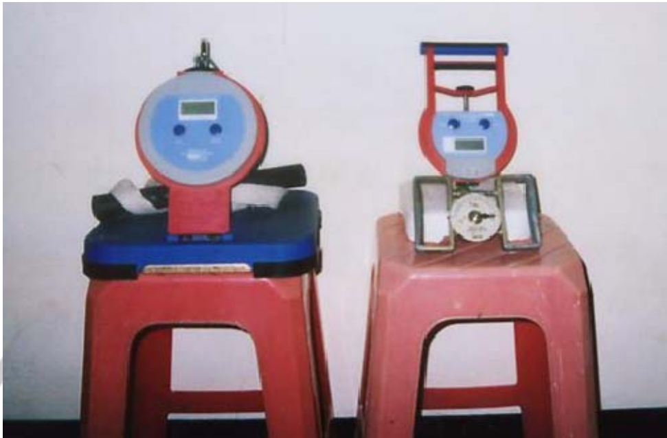
Gambar 1 : Back and Leg Dynamometer , Pull and Push Dynamometer dan Grip Strength Dynamometer
