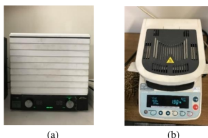
Fig. 1: (a) The use of a tool Drying Machine (Dryer code TTM-440N by Akira Higashi, Japan) (b) Device for Analysing Moisture (MF-50 production of AND company)
