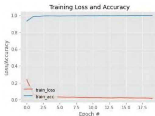
Figure 5. Training loss vs. accuracy classifier
