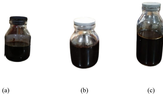
Gambar 1. Produk Bio-Oil Hasil Pirolisis TKKS; (a) Laju Alir Nitrogen 1 L/min; (b) Laju Alir Nitrogen 2 L/min; (c) Laju Alir Nitrogen 3 L/min
