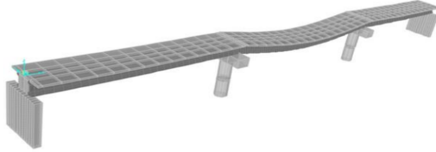
(a) Bending vertical mode 1st
