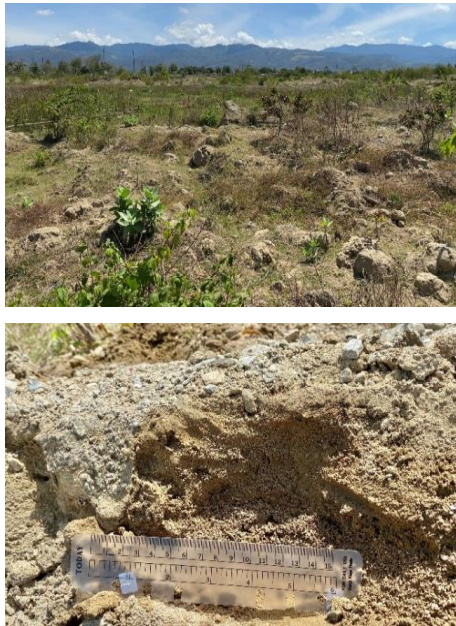
Figure 5. Wide-spread liquefied soils on the surface of Petobo slide: (up) general view, (down) close view; during 02/2020 site reconnaissance (Kusumawardani et al., 2021).
