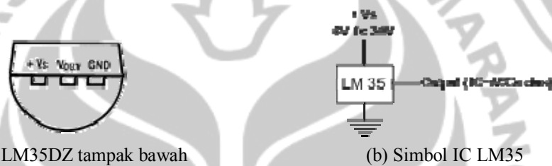
Gambar 2.1 Sensor suhu IC LM35DZ (Datasheet LM35, 2000)
