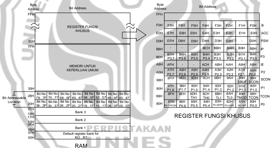
Gambar 2.10 Peta memori data internal AT89S51
