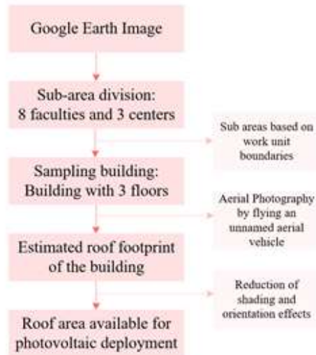
Figure 4. Identification of building samples and estimation of roof area
