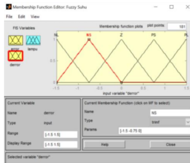
Figure 2. Temperature Membership Function Derror
