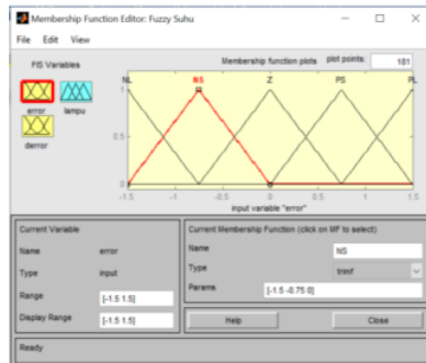
Figure 1. Temperature Membership Function Error
