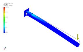
Figure 8. Von mises stress
