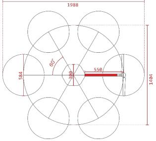
Figure 2. Sketch 2D drone dimension size
