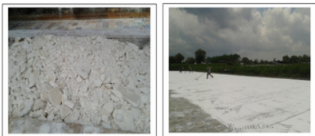
Figure 11a. Wet Krosok without drying, and 11b. Tapioca Drying Process
