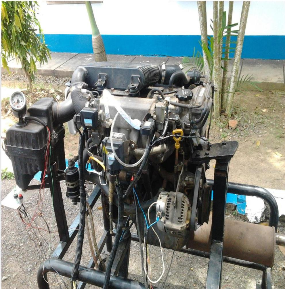
Foto *Engine stand* mesin Starlet GT Turbo EFI 4E-FTE
