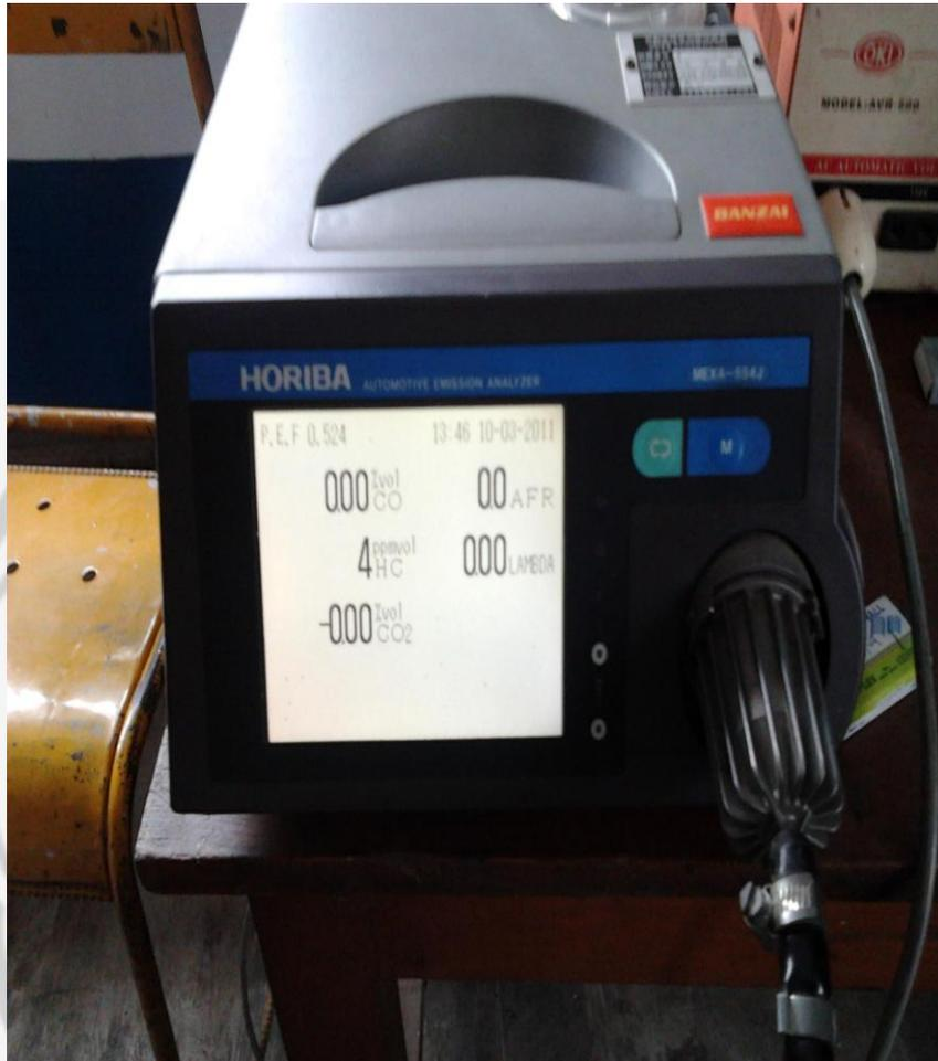
Foto Alat Horiba *Automotive Analyzer* seri mexa-554J
