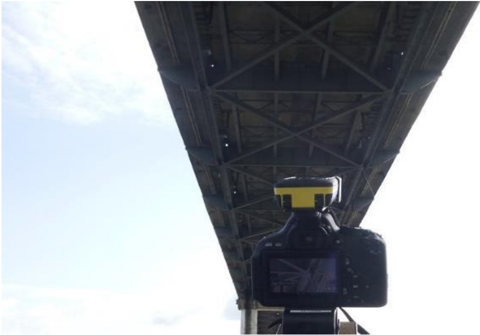
Figure 7. Deflection measurement from the ground
