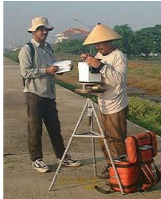
Figure 1. Measurement of gravity vertical gradient
