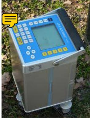
**Gambar 2. Gravometer Scintrex Autograv CG-5**
