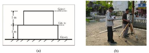
**Figure 1.** (a) Schematic model of gravity measurements to determine the vertical gradient and (b) measurement of the vertical gradient of gravity
