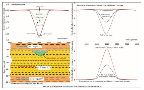
Figure 3. Characteristics of micro-gravity vertical gradient over time due to the replenishment of groundwater
