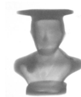
Figure 4. Phantom image with exposure factors of 50kV, 0.2 s and 16 mA.
