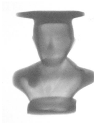
Figure 4. Phantom image with exposure factors of 50kV, 0.2 s and 16 mA.
