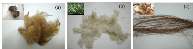
Figure 2. Fiber separation results: (a) Areca nut skin fiber, (b) Pineapple leaf fiber, and (c) Coconut fiber.
