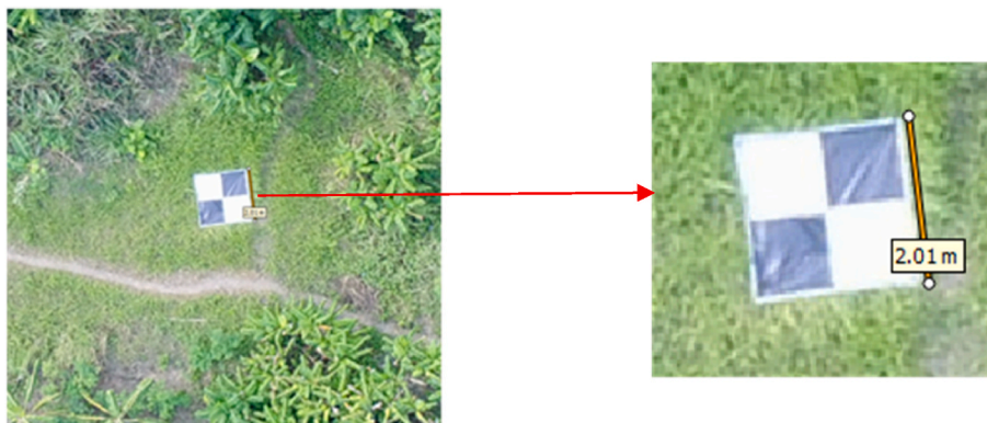
Fig. 5. The accuracy of the image from UAV acquisition with GCP.
