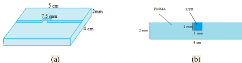
Figure 1. (a) Design of cladding (b) Cross section of the waveguide
