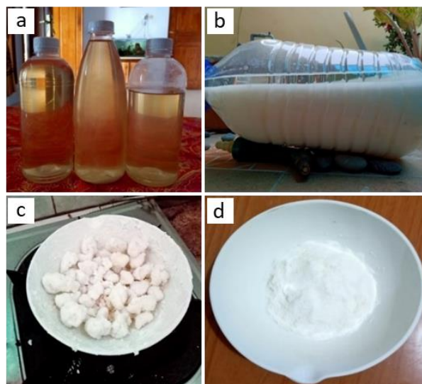
Figure 2. (a) bittern sample from PT. Garam Mas, Rembang (b) precipitation process (c) agglomeration of \text{Mg}(\text{OH})_2 (d) synthesis result
