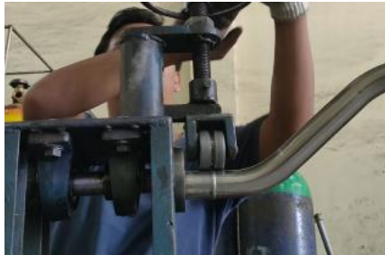
Gambar 6.16 Proses forming garis timbul
