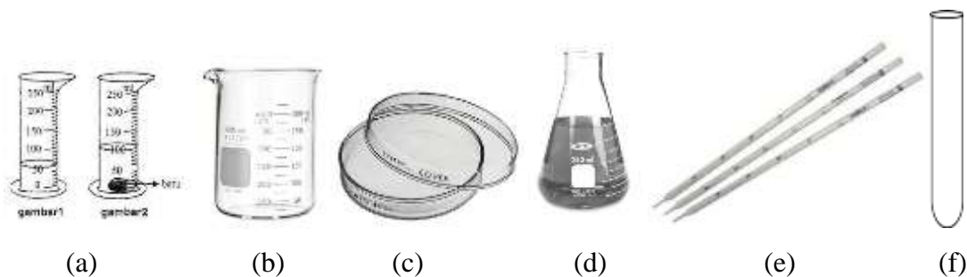
Gambar 1.1 (a) gelas ukur, (b) Beaker glass, (c) petridish, (d) erlenmeyer, (e) pipet ukur, (f) tabung reaksi
