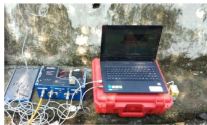
FIGURE 4. The Sensor is connected to the recorder that already connected to the laptop.
