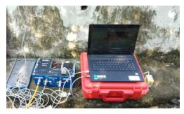
FIGURE 4. The Sensor is connected to the recorder that already connected to the laptop.
