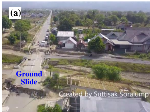
Fig. 18 Morphological features observed from the snapshots of drone videos by Soralump (2018). a Photo of the ground slide feature along Moh. Soeharto road to the east boundary of Petobo slide (facing east). b Photo of the features of liquefaction spread, liquefaction flow, and debris flood on the south-eastern portion of Petobo slide (facing west).
