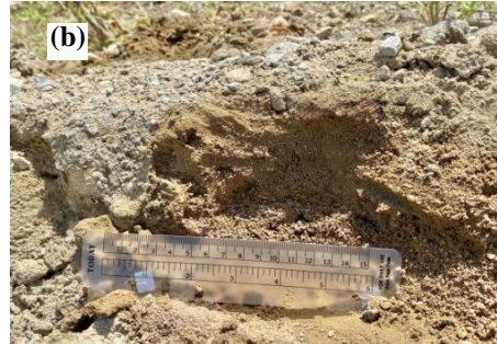
Fig. 8 a. A site with big eruptions of sands during earthquake based on the interviews with Witnesses G and H. The location was near District Office of Petobo (Kantor Kelurahan Petobo). b, c Exposed sands as evidences of soil liquefaction.
