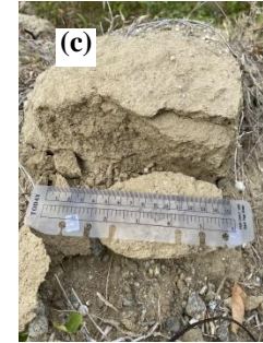
Fig. 8 a. A site with big eruptions of sands during earthquake based on the interviews with Witnesses G and H. The location was near District Office of Petobo (Kantor Kelurahan Petobo). b, c Exposed sands as evidences of soil liquefaction.
