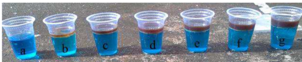
Fig. 1. (a). Methylene blue solution and methylene blue solution with catalyst C-Dots : (b). 10 mL, (c). 20 mL, (d). 30 mL, (e). 40 mL, (f). 50 mL and (g). 60 mL
