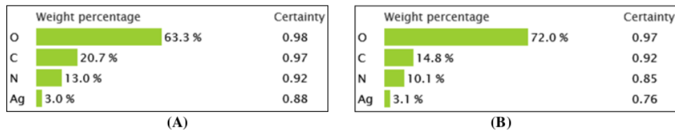
Figure 4 The weight percentage of Ag, N, C, O in the transparent spot (A) and dark spot (B)
