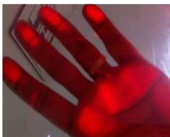
Figure 2: pressure at the sensor breaks down total internal reflection & scatters its beams downwards
