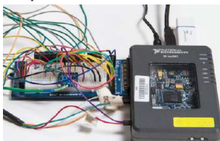
Figure.4. Hardware connection of 18B20 temperature sensor
