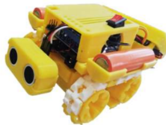
Figure 2. The SMARS robot after it is completely assembled
