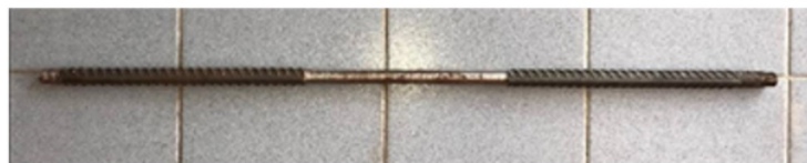
(b) The actual size of fuse bar and 13mm diameter at middle part after trimming it.
