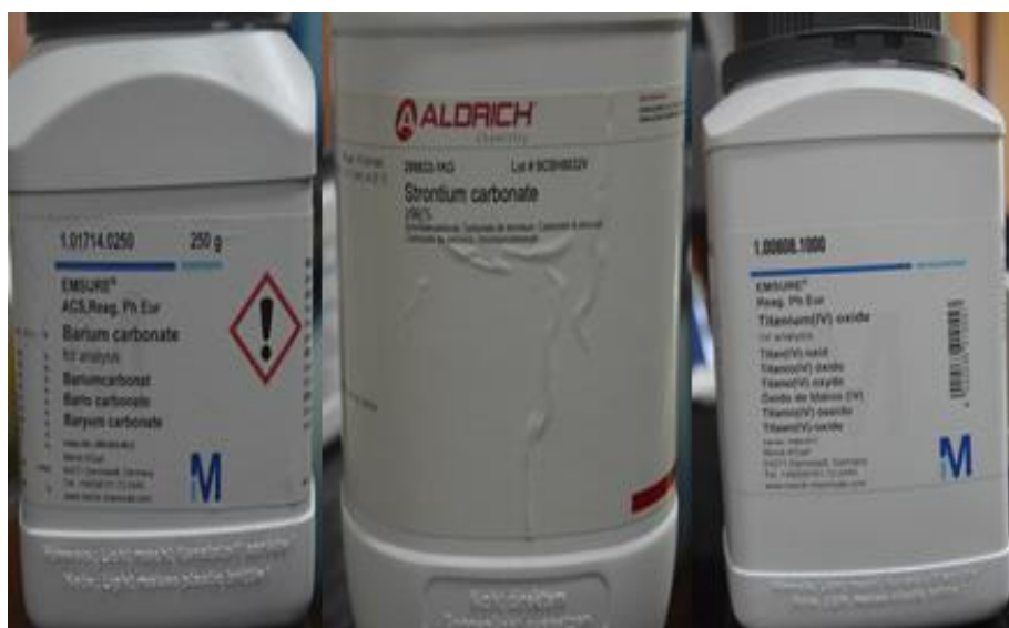
Figure 1. Powder of \text{BaCO}_3 , \text{SrCO}_3 and \text{TiO}_2 as The Raw Material for synthesis \text{Ba}_{0.6}\text{Sr}_{0.4}\text{TiO}_3 material
