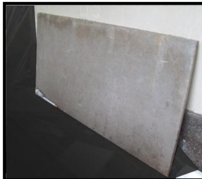
Figure 2. Application of cement particle board as a form of house (Source: Researcher, 2010).
