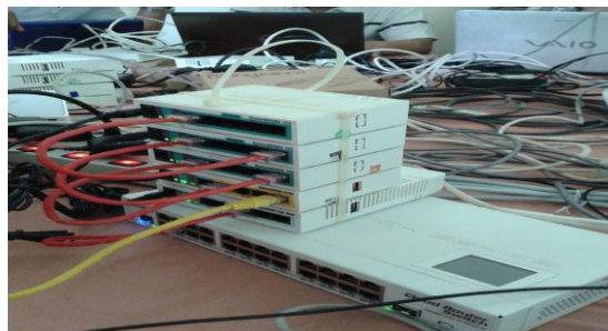
Figure 3 Lab routing OSPF with RouterMikrotik
