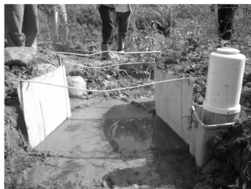
Fig. 2 The Parshall flume used in the experiment.
