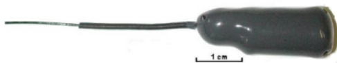
Frequency range : 138 to 235 MHz Transmitter : Crystal controlled two stage design, pulse by CMOS multivibrator
