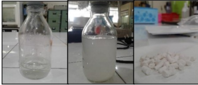
Figure 2. Silica precipitation (Process condition: washed with 1 mol/L HCl solution, extracted with 1 mol/L NaOH, ratio of SCBA:NaOH = 1:10 w/v, volume = 100 mL; precipitated with 1 mol/L HCl solution).
