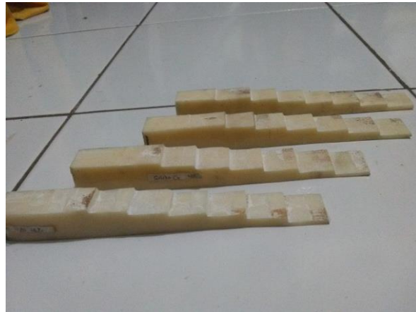
Figure 1. Stepwedge of Resin- \text{Al}_2\text{O}_3 and Resin- \text{SiO}_2
