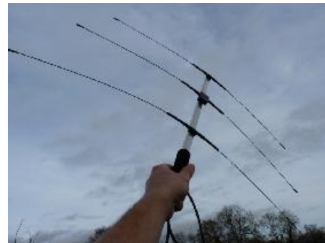
Figure 3 Antenna Yagi 151 MHz
