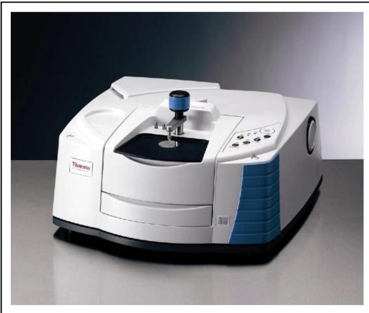
**Gambar 3.20.** FTIR spectrometer
