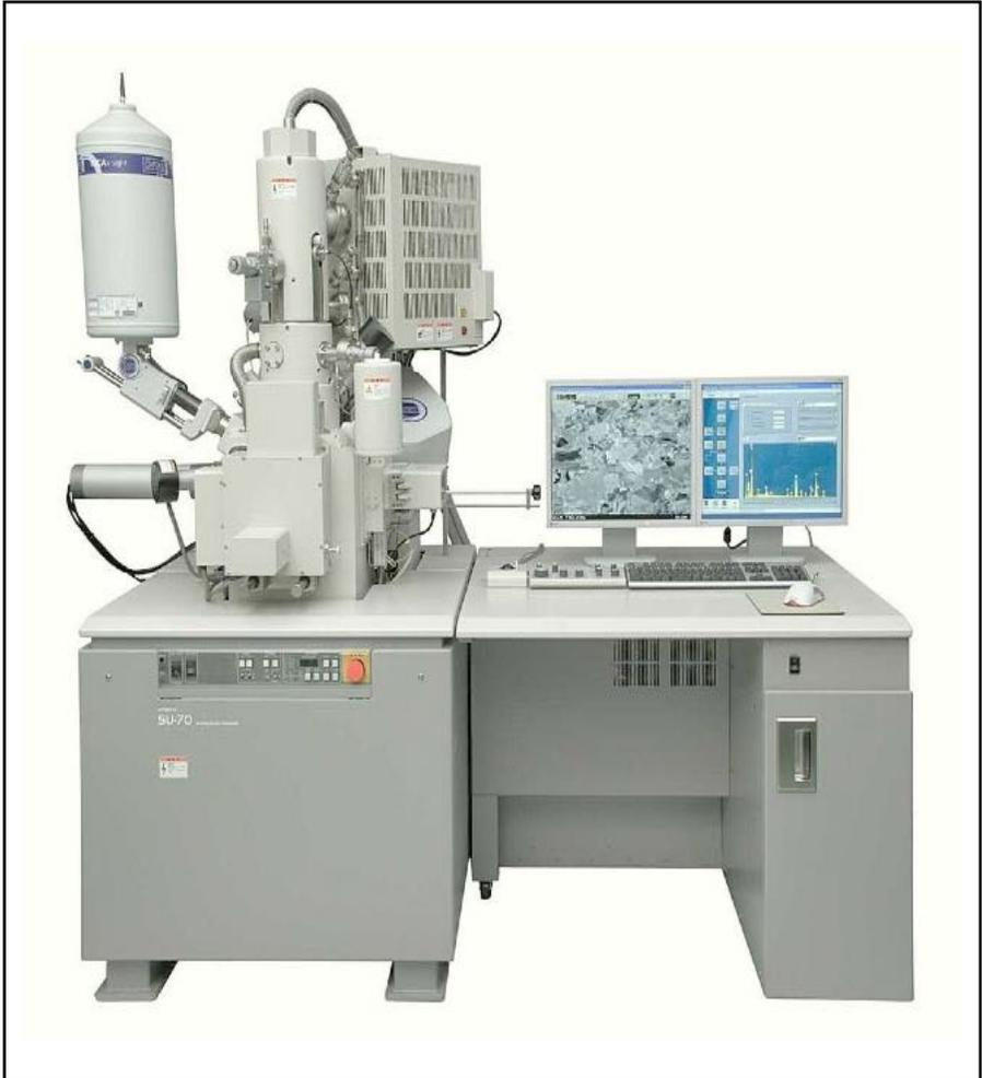
**Gambar 3.12.** Alat *scanning electron microscope*
