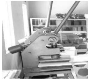
Figure 4 The pressing-cutting process of evafoam
