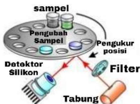
Gambar 2.7 Prinsip X-Ray Fluorescence
