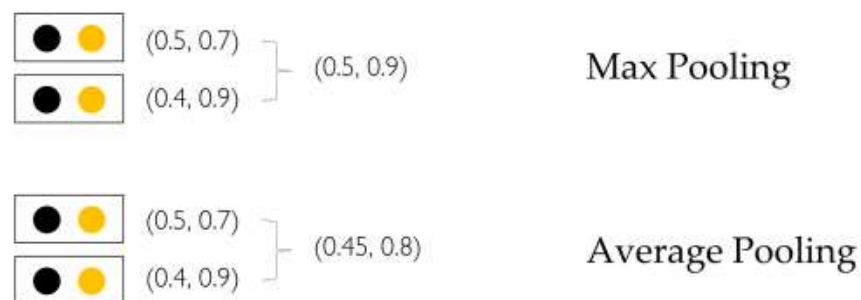
Gambar 2.15 Max Pooling dan Average Pooling
